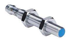
Contrinex inductive proximity sensor, tubular, 8mm diameter x 60mm body, chrome-plated nickel silver housing, NPN, N.O. output, 4mm sensing distance, semi-flush, 500 Hz switching frequency, IP67, 3-pin M8 quick-disconnect.
