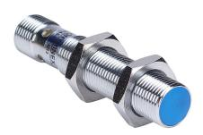
Contrinex inductive proximity sensor, tubular, 12mm diameter x 60mm body, chrome-plated brass housing, NPN, N.O. output, 8mm sensing distance, semi-flush, 400 Hz switching frequency, IP67, 4-pin M12 quick-disconnect.
