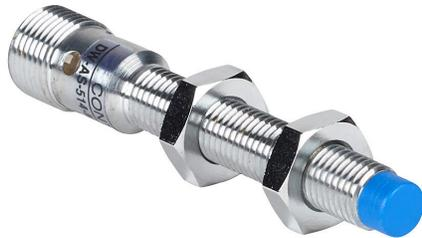
Contrinex inductive proximity sensor, tubular, 8mm diameter x 66mm body, chrome-plated brass housing, PNP, N.C. output, 6mm sensing distance, non-flush, 500 Hz switching frequency, IP67, 4-pin M12 quick-disconnect.
