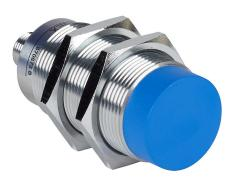
Contrinex inductive proximity sensor, tubular, 30mm diameter x 73.5mm body, chrome-plated brass housing, PNP, N.C. output, 40mm sensing distance, non-flush, 100 Hz switching frequency, IP67, 4-pin M12 quick-disconnect.
