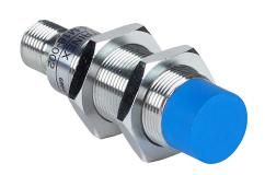
Contrinex inductive proximity sensor, tubular, 18mm diameter x 63.5mm body, chrome-plated brass housing, PNP, N.C. output, 20mm sensing distance, non-flush, 500 Hz switching frequency, IP67, 4-pin M12 quick-disconnect.
