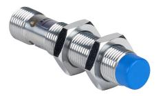
Contrinex inductive proximity sensor, tubular, 12mm diameter x 60mm body, chrome-plated brass housing, PNP, N.C. output, 10mm sensing distance, non-flush, 400 Hz switching frequency, IP67, 4-pin M12 quick-disconnect.
