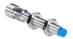
Contrinex inductive proximity sensor, tubular, 8mm diameter x 66mm body, chrome-plated brass housing, PNP, N.O. output, 6mm sensing distance, non-flush, 500 Hz switching frequency, IP67, 4-pin M12 quick-disconnect.
