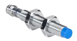
Contrinex inductive proximity sensor, tubular, 8mm diameter x 60mm body, chrome-plated brass housing, PNP, N.O. output, 6mm sensing distance, non-flush, 500 Hz switching frequency, IP67, 3-pin M8 quick-disconnect.
