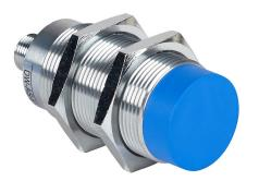
Contrinex inductive proximity sensor, tubular, 30mm diameter x 73.5mm body, chrome-plated brass housing, PNP, N.O. output, 40mm sensing distance, non-flush, 100 Hz switching frequency, IP67, 4-pin M12 quick-disconnect.
