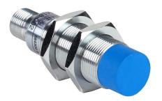
Contrinex inductive proximity sensor, tubular, 18mm diameter x 63.5mm body, chrome-plated brass housing, PNP, N.O. output, 20mm sensing distance, non-flush, 500 Hz switching frequency, IP67, 4-pin M12 quick-disconnect.
