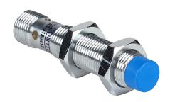
Contrinex inductive proximity sensor, tubular, 12mm diameter x 60mm body, chrome-plated brass housing, PNP, N.O. output, 10mm sensing distance, non-flush, 400 Hz switching frequency, IP67, 4-pin M12 quick-disconnect.
