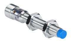
Contrinex inductive proximity sensor, tubular, 8mm diameter x 66mm body, chrome-plated brass housing, NPN, N.C. output, 6mm sensing distance, non-flush, 500 Hz switching frequency, IP67, 4-pin M12 quick-disconnect.
