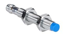
Contrinex inductive proximity sensor, tubular, 8mm diameter x 60mm body, chrome-plated brass housing, NPN, N.C. output, 6mm sensing distance, non-flush, 500 Hz switching frequency, IP67, 3-pin M8 quick-disconnect.
