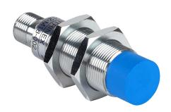
Contrinex inductive proximity sensor, tubular, 18mm diameter x 63.5mm body, chrome-plated brass housing, NPN, N.C. output, 20mm sensing distance, non-flush, 500 Hz switching frequency, IP67, 4-pin M12 quick-disconnect.
