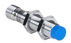
Contrinex inductive proximity sensor, tubular, 12mm diameter x 60mm body, chrome-plated brass housing, NPN, N.C. output, 10mm sensing distance, non-flush, 400 Hz switching frequency, IP67, 4-pin M12 quick-disconnect.
