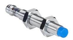
Contrinex inductive proximity sensor, tubular, 8mm diameter x 60mm body, chrome-plated brass housing, NPN, N.O. output, 6mm sensing distance, non-flush, 500 Hz switching frequency, IP67, 3-pin M8 quick-disconnect.
