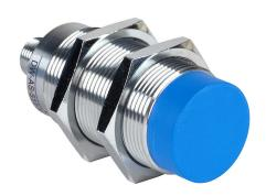
Contrinex inductive proximity sensor, tubular, 30mm diameter x 73.5mm body, chrome-plated brass housing, NPN, N.O. output, 40mm sensing distance, non-flush, 100 Hz switching frequency, IP67, 4-pin M12 quick-disconnect.
