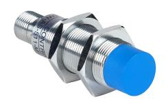
Contrinex inductive proximity sensor, tubular, 18mm diameter x 63.5mm body, chrome-plated brass housing, NPN, N.O. output, 20mm sensing distance, non-flush, 500 Hz switching frequency, IP67, 4-pin M12 quick-disconnect.
