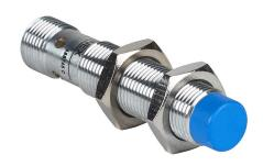
Contrinex inductive proximity sensor, tubular, 12mm diameter x 60mm body, chrome-plated brass housing, NPN, N.O. output, 10mm sensing distance, non-flush, 400 Hz switching frequency, IP67, 4-pin M12 quick-disconnect.
