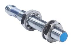
Contrinex inductive proximity sensor, tubular, 8mm diameter x 60mm body, chrome-plated brass housing, 0-10 VDC analog output, 4mm sensing distance, semi-flush, IP67, 3-pin M8 quick-disconnect.
