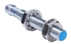
Contrinex inductive proximity sensor, tubular, 8mm diameter x 60mm body, chrome-plated brass housing, 0-5 VDC analog output, 4mm sensing distance, semi-flush, IP67, 3-pin M8 quick-disconnect.
