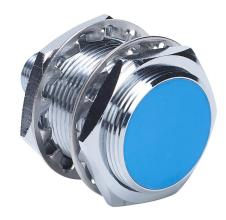
Contrinex inductive proximity sensor, tubular, 30mm diameter x 48.5mm body, chrome-plated brass housing, 0-10 VDC or 4-20 mA analog output, 20mm sensing distance, semi-flush, IP67, 4-pin M12 quick-disconnect.
