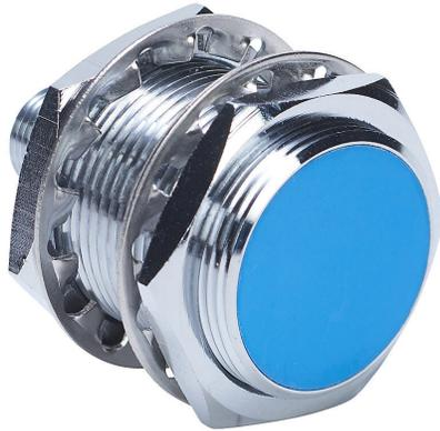
Contrinex inductive proximity sensor, tubular, 30mm diameter x 48.5mm body, chrome-plated brass housing, 0-10 VDC or 4-20 mA analog output, 20mm sensing distance, semi-flush, IP67, 4-pin M12 quick-disconnect.
