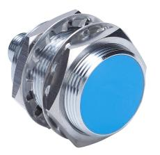
Contrinex inductive proximity sensor, tubular, 30mm diameter x 48.5mm body, chrome-plated brass housing, 0-5 VDC or 1-5 mA analog output, 20mm sensing distance, semi-flush, IP67, 4-pin M12 quick-disconnect.
