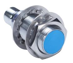
Contrinex inductive proximity sensor, tubular, 18mm diameter x 48.5mm body, chrome-plated brass housing, 0-10 VDC or 4-20 mA analog output, 10mm sensing distance, semi-flush, IP67, 4-pin M12 quick-disconnect.
