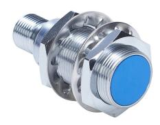
Contrinex inductive proximity sensor, tubular, 18mm diameter x 48.5mm body, chrome-plated brass housing, 0-5 VDC or 1-5 mA analog output, 10mm sensing distance, semi-flush, IP67, 4-pin M12 quick-disconnect.
