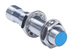
Contrinex inductive proximity sensor, tubular, 12mm diameter x 60mm body, chrome-plated brass housing, 0-5 VDC or 1-5 mA analog output, 6mm sensing distance, semi-flush, IP67, 4-pin M12 quick-disconnect.
