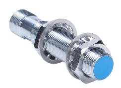
Contrinex inductive proximity sensor, tubular, 12mm diameter x 60mm body, chrome-plated brass housing, 0-10 VDC or 4-20 mA analog output, 6mm sensing distance, semi-flush, IP67, 4-pin M12 quick-disconnect.
