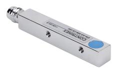
Contrinex inductive proximity sensor, rectangular, 8 x 8 x 59mm body, chrome-plated brass housing, 0-10 VDC analog output, 4mm sensing distance, semi-flush, IP67, 3-pin M8 quickdisconnect.
