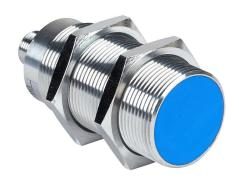
Contrinex inductive proximity sensor, tubular, 30mm diameter x 73.5mm body, chrome-plated brass housing, PNP, N.C. output, 22mm sensing distance, semi-flush, 200 Hz switching frequency, IP67, 4-pin M12 quick-disconnect.
