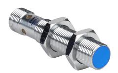
Contrinex inductive proximity sensor, tubular, 12mm diameter x 60mm body, chrome-plated brass housing, PNP, N.C. output, 6mm sensing distance, semi-flush, 800 Hz switching frequency, IP67, 4-pin M12 quick-disconnect.
