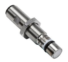
Contrinex inductive proximity sensor, tubular, 12mm diameter x 56mm body, 304 stainless steel housing, PNP, N.O., 1.5mm sensing distance, flush, 600 Hz switching frequency, IP68, 4-pin M12 quick-disconnect.
