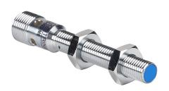
Contrinex inductive proximity sensor, tubular, 8mm diameter x 66mm body, chrome-plated nickel silver housing, PNP, N.O. output, 3mm sensing distance, semi-flush, 1 kHz switching frequency, IP67, 4-pin M12 quick-disconnect.
