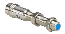
Contrinex inductive proximity sensor, tubular, 5mm diameter x 38mm body, nickel silver housing, PNP, N.O. output, 2.5mm sensing distance, semi-flush, 800 Hz switching frequency, IP67, 3-pin M8 quick-disconnect.
