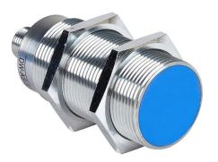
Contrinex inductive proximity sensor, tubular, 30mm diameter x 73.5mm body, chrome-plated brass housing, PNP, N.O. output, 22mm sensing distance, semi-flush, 200 Hz switching frequency, IP67, 4-pin M12 quick-disconnect.
