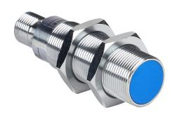
Contrinex inductive proximity sensor, tubular, 18mm diameter x 63.5mm body, chrome-plated brass housing, PNP, N.O. output, 12mm sensing distance, semi-flush, 600 Hz switching frequency, IP67, 4-pin M12 quick-disconnect.
