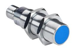
Contrinex inductive proximity sensor, tubular, 18mm diameter x 63.5mm body, chrome-plated brass housing, PNP, N.O. output, 12mm sensing distance, semi-flush, 600 Hz switching frequency, IP67, 4-pin M12 quick-disconnect.
