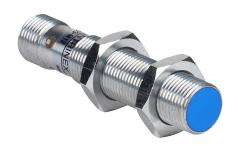
Contrinex inductive proximity sensor, tubular, 12mm diameter x 60mm body, chrome-plated brass housing, PNP, N.O. output, 6mm sensing distance, semi-flush, 800 Hz switching frequency, IP67, 4-pin M12 quick-disconnect.
