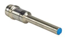
Contrinex inductive proximity sensor, tubular, 4mm diameter x 38mm body, nickel silver housing, PNP, N.O. output, 2.5mm sensing distance, semi-flush, 800 Hz switching frequency, IP67, 3-pin M8 quick-disconnect.
