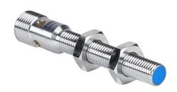
Contrinex inductive proximity sensor, tubular, 8mm diameter x 66mm body, chrome-plated nickel silver housing, NPN, N.C. output, 3mm sensing distance, semi-flush, 1 kHz switching frequency, IP67, 4-pin M12 quick-disconnect.
