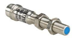
Contrinex inductive proximity sensor, tubular, 5mm diameter x 38mm body, nickel silver housing, NPN, N.C. output, 2.5mm sensing distance, semi-flush, 800 Hz switching frequency, IP67, 3-pin M8 quick-disconnect.
