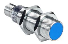
Contrinex inductive proximity sensor, tubular, 18mm diameter x 63.5mm body, chrome-plated brass housing, NPN, N.C. output, 12mm sensing distance, semi-flush, 600 Hz switching frequency, IP67, 4-pin M12 quick-disconnect.
