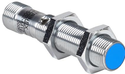
Contrinex inductive proximity sensor, tubular, 12mm diameter x 60mm body, chrome-plated brass housing, NPN, N.C. output, 6mm sensing distance, semi-flush, 800 Hz switching frequency, IP67, 4-pin M12 quick-disconnect.
