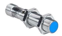
Contrinex inductive proximity sensor, tubular, 12mm diameter x 60mm body, chrome-plated brass housing, NPN, N.C. output, 6mm sensing distance, semi-flush, 800 Hz switching frequency, IP67, 4-pin M12 quick-disconnect.
