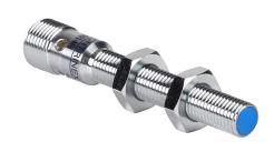
Contrinex inductive proximity sensor, tubular, 8mm diameter x 66mm body, chrome-plated nickel silver housing, NPN, N.O. output, 3mm sensing distance, semi-flush, 1 kHz switching frequency, IP67, 4-pin M12 quick-disconnect.
