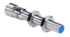
Contrinex inductive proximity sensor, tubular, 8mm diameter x 66mm body, chrome-plated nickel silver housing, NPN, N.O. output, 3mm sensing distance, semi-flush, 1 kHz switching frequency, IP67, 4-pin M12 quick-disconnect.
