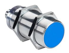
Contrinex inductive proximity sensor, tubular, 30mm diameter x 73.5mm body, chrome-plated brass housing, NPN, N.O. output, 22mm sensing distance, semi-flush, 200 Hz switching frequency, IP67, 4-pin M12 quick-disconnect.
