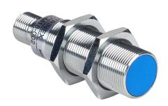
Contrinex inductive proximity sensor, tubular, 18mm diameter x 63.5mm body, chrome-plated brass housing, NPN, N.O. output, 12mm sensing distance, semi-flush, 600 Hz switching frequency, IP67, 4-pin M12 quick-disconnect.
