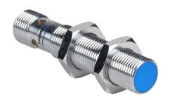
Contrinex inductive proximity sensor, tubular, 12mm diameter x 60mm body, chrome-plated brass housing, NPN, N.O. output, 6mm sensing distance, semi-flush, 800 Hz switching frequency, IP67, 4-pin M12 quick-disconnect.
