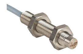
Contrinex inductive proximity sensor, tubular, 8mm diameter x 45mm body, stainless steel housing, PNP, N.C. output, 6mm sensing distance, non-flush, 700 Hz switching frequency, IP67 IP68, pigtail.
