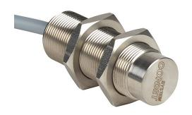
Contrinex inductive proximity sensor, tubular, 18mm diameter x 50mm body, stainless steel housing, PNP, N.C. output, 20mm sensing distance, non-flush, 200 Hz switching frequency, IP68 IP69K, pigtail.
