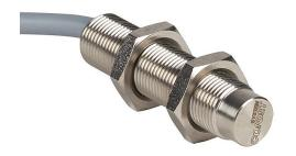
Contrinex inductive proximity sensor, tubular, 12mm diameter x 50mm body, stainless steel housing, PNP, N.C. output, 10mm sensing distance, non-flush, 400 Hz switching frequency, IP68 IP69K, pigtail.
