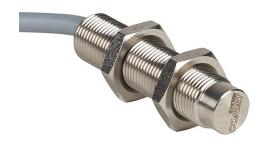
Contrinex inductive proximity sensor, tubular, 12mm diameter x 50mm body, stainless steel housing, PNP, N.C. output, 10mm sensing distance, non-flush, 400 Hz switching frequency, IP68 IP69K, pigtail.
