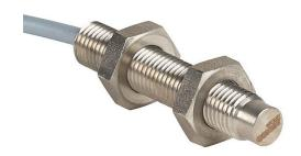
Contrinex inductive proximity sensor, tubular, 8mm diameter x 45mm body, stainless steel housing, PNP, N.O. output, 6mm sensing distance, non-flush, 700 Hz switching frequency, IP67 IP68, pigtail.
