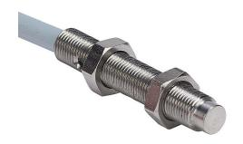
Contrinex inductive proximity sensor, tubular, 5mm diameter x 30mm body, stainless steel housing, PNP, N.O. output, 3mm sensing distance, non-flush, 1.2 kHz switching frequency, IP67, pigtail.
